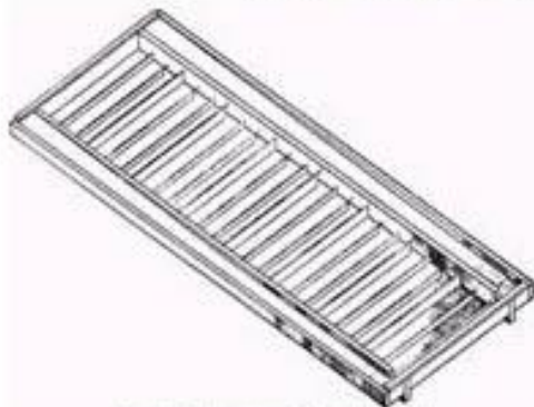
Figure 4—Evaporator with skimming trough
